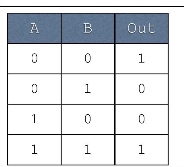
Idea: for every output in the truth table which has a 1, write an AND which corresponds to it
