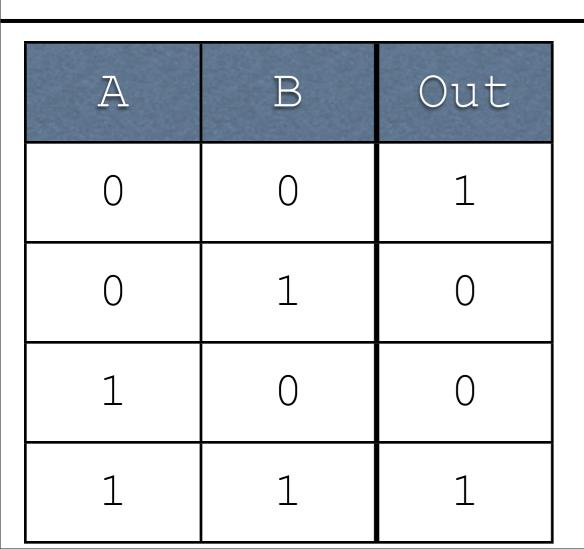
Idea: for every output in the truth table which has a 1, write an AND which corresponds to it
