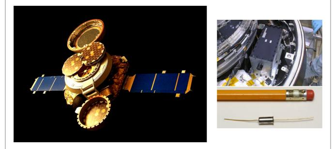
Accelerometer installed backwards leads to three year loss. Test which would have caught it was skipped.
